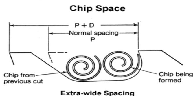
Gullet is provided to accommodate the chips formed during the broaching by each of teeth which cannot escape until the enclosing adjacent teeth have cleared the component. Chip space is limited by the pitch of the tooth and in small diameter broaches.
